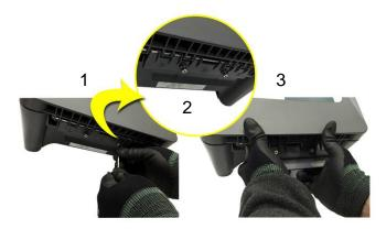
Figure 9. Undoing the Two Security Screws and Opening the Enclosure
