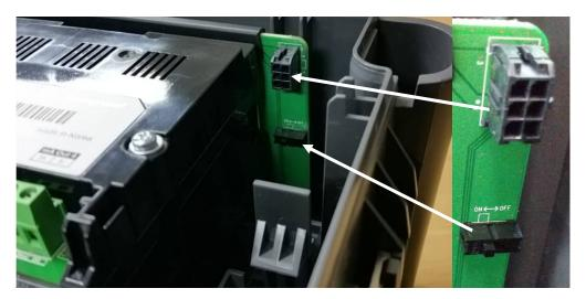
Figure 18. Battery On/Off Switch and Battery Connector
